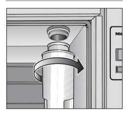
■ Screw the salt container firmly onto the socket.
